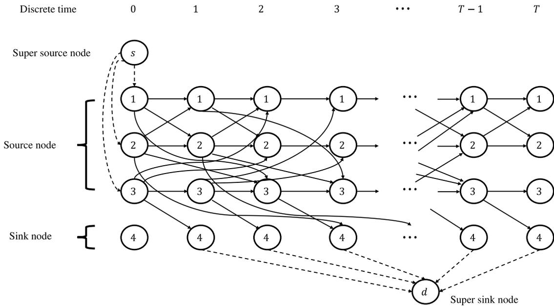
Fig. 2. Example of converting a static network into a dynamic network by introducing a super source node and a super sink node [16].
