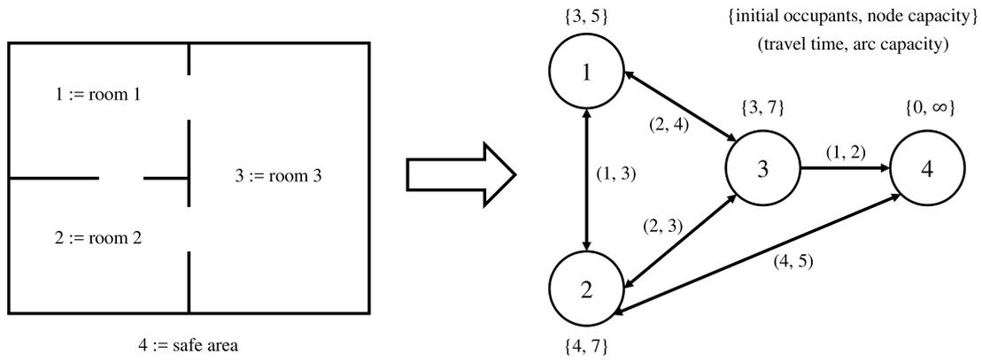
Fig. 1. Example of converting the structure of a building to a network  $G = (\mathcal{N}, \mathcal{A})$  [16].
